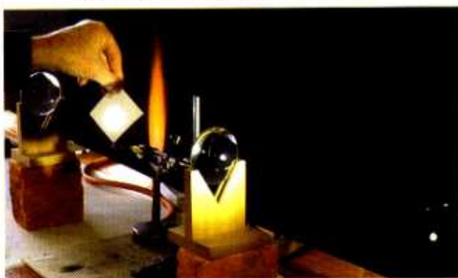
Fig.3 Photograph of the apparatus looking towards the white-light Lumiled. Note how little peripheral light is emitted from the source when the viewpoint lies only a few degrees off axis. The lenses in the photograph have diameters of 75 mm, whereas the ones recommended in the text are 50 mm.
