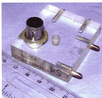
Figure 2 The Panax collimated sealed source (Type S4). The dose rate is rather high with the collimator removed.
