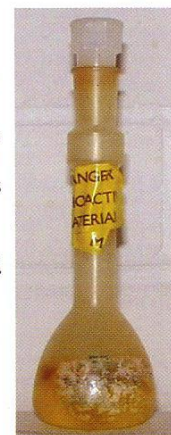
Figure 4 School-made protactinium generator, to SSERC design.
