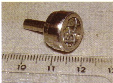
Figure 1 Sealed source – a type of source made by Amersham, in widespread use.
