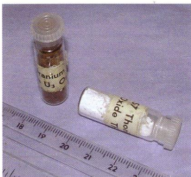
Figure 7 Orphan sources - Panax open sources (Types S6 and S7, uranium and thorium oxide) – examples of orphan sources that should have been disposed of in the 1980s, but whose disposal is now inordinately difficult to arrange.
