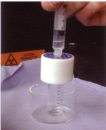
Figure 5 Eluting the short-lived radionuclide Barium-137m from the Isotope Generator.
