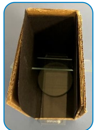
Figure 10 - Newton's rings apparatus made from cardboard and two microscope slides.
