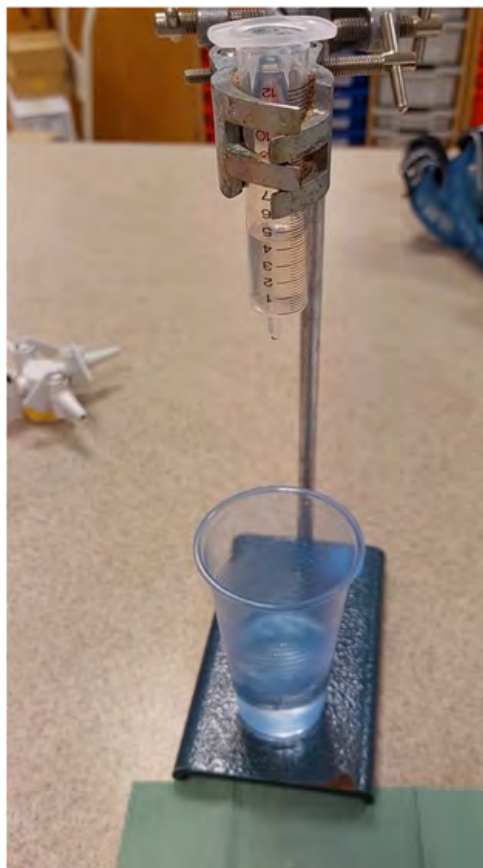
Figure 6: Steps in preparing immobilised algae. The barrel of a 10 cm 3 syringe is clamped into a retort stand, positioned above a container of 2% calcium chloride. The mixture of algae and sodium alginate is transferred into the barrel of the syringe and allowed to drop into the calcium chloride. As the drop makes contact with the calcium chloride, it forms a bead, which continues to harden over time. Allow approximately 5 minutes after beads have been produced before thoroughly rinsing with distilled water.
