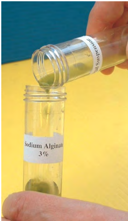
Figure 6: Steps in preparing immobilised algae. The barrel of a 10 cm 3 syringe is clamped into a retort stand, positioned above a container of 2% calcium chloride. The mixture of algae and sodium alginate is transferred into the barrel of the syringe and allowed to drop into the calcium chloride. As the drop makes contact with the calcium chloride, it forms a bead, which continues to harden over time. Allow approximately 5 minutes after beads have been produced before thoroughly rinsing with distilled water.
