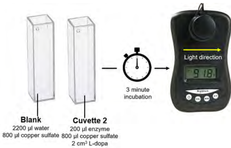
Figure 4: Integrated diagram to show assay to test the effect of copper sulfate on dopa oxidase activity. Copper sulfate has published inhibitory effects on dopa oxidase and, as such, provides a positive control for this investigation. The colorimetric blank must include the same proportion of copper sulfate as in the test sample (cuvette 2) to account for the colour of the solution.
