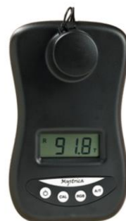
Figure 2. To measure the transmission of light through the enzyme-treated apple juice. Prepare the colorimetric blank to account for the effect of the coloured enzyme solution. Then decant the supernatant from each of the reactions into separate cuvettes. Measure the transmission of light through the samples using the blue diode.
