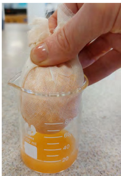
Figure 4: This procedure allows the extraction of beta-amylase (enzyme) from sweet potato. A 30 g sample of sweet potato is cut, blended and then passed through muslin. The collected liquid contains the enzyme and can be stored.
