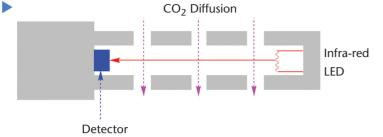
Figure 3 - Schematic representation of the Vernier CO<sub>2</sub> gas sensor.
